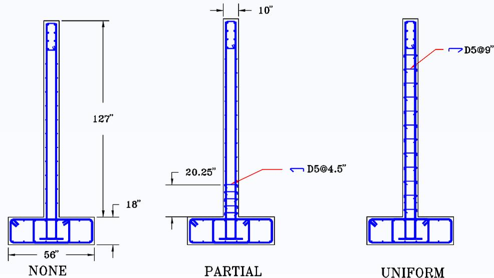
Lap splices at the bottom of the wall in the plastic hinge zone degrades the performance and ductility of the wall. Thus, it is recommended to avoid using splices in the plastic hinge zone, or welded splices should be used
